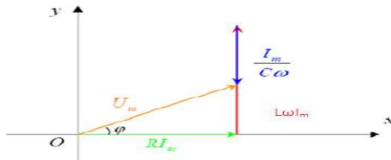
Théorème de Pythagore:  $U_m^2 = (R I_m)^2 + \left(L \omega I_m - \frac{I_m}{C \omega}\right)^2 \Rightarrow U_m = I_m \sqrt{R^2 + \left(L \omega - \frac{1}{C \omega}\right)^2}$  d'où
